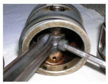
They are HT (very) and by choosing a 'cap head' I could use a straight Allen-key to get outside the skirt and apply my torque wrench via a series of adaptors.
